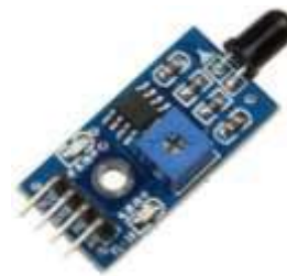
Fig No.07 Fire sensor
