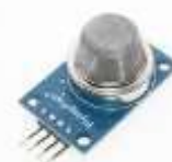
Fig No.09 Smoke Sensor
